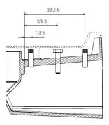
Section : Housing Bolt / Screw Layout
