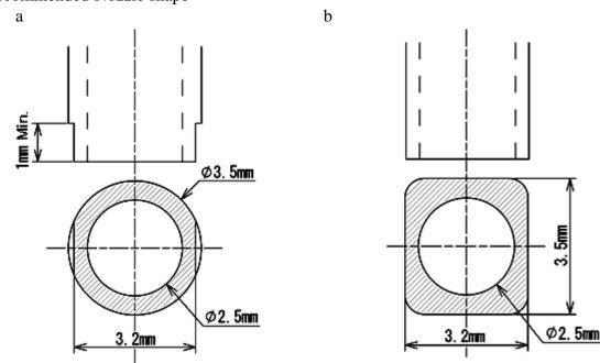
\*Nozzle with chamfering is recommended
