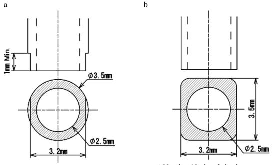
\*Nozzle with chamfering is recommended
