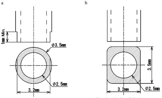
\*Nozzle with chamfering is recommended
