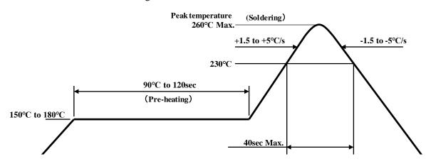
Note 1 Temperature profile for the reflow should be set to the surface temperature of resin which is on the top of LED. This should be the maximum temperature for soldering. Lowering the heating temperature and decreasing heating time is very effective in achieving higher reliability.
