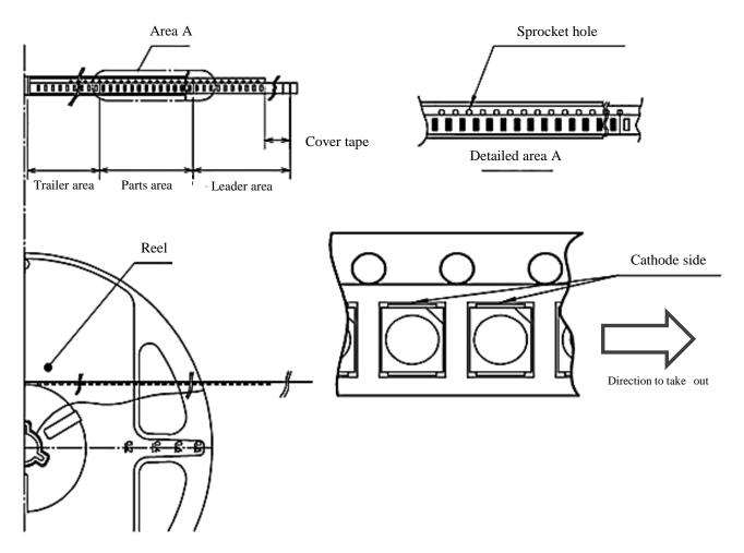
Note "-TR" means Cathode Side of LEDs; should be placed on the sprocket-hole side.
