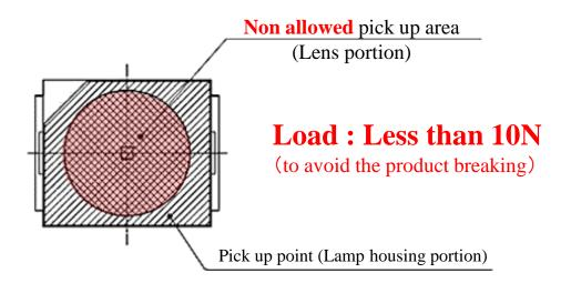
Please adjust the load, the pick up point, the nozzle diameter and etc. before mounting because the over load can cause the breakage of the lamp housing.
