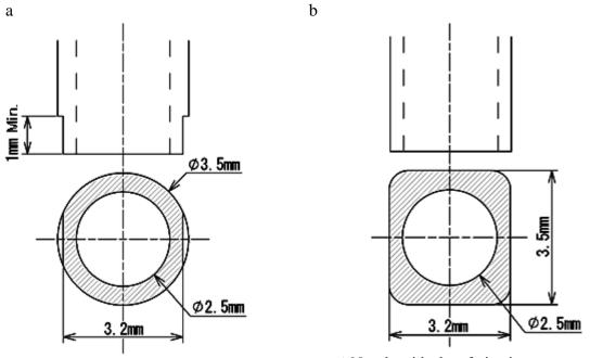
\*Nozzle with chamfering is recommended
