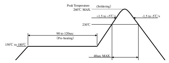
Note 1 Temperature profile for the reflow should be set to the surface temperature of resin which is on the top of LED. This should be the maximum temperature for soldering. Lowering the heating temperature and decreasing heating time is very effective in achieving higher reliability.
