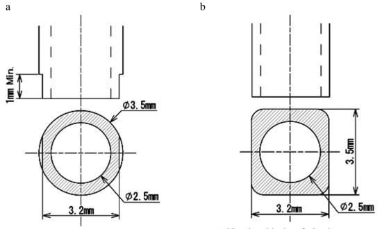
\*Nozzle with chamfering is recommended
