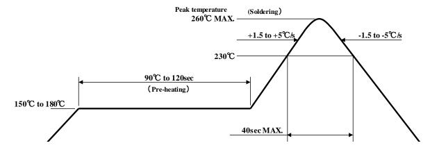
Notes 1 Temperature Profile for the reflow should be set to the surface temperature of resin which is on the top of LED. This should be the maximum temperature for soldering. Lowering the heating temperature and decreasing heating time is very effective in achieving higher reliability.
