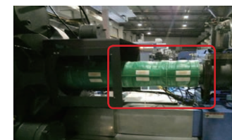
Red outlined section: Countermeasures against heat loss
